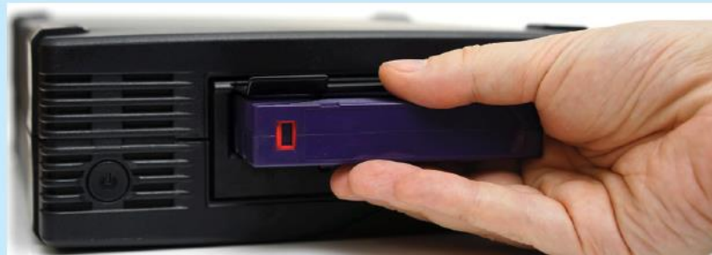
Figure 11.5 An LTO-6 Tape drive with tape cartridge inserted.
