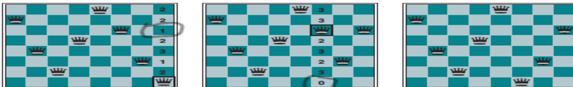
Figure 5.8 A two-step solution using min-conflicts for an 8-queens problem. At each stage, a queen is chosen for reassignment in its column. The number of conflicts (in this case, the number of attacking queens) is shown in each square. The algorithm moves the queen to the min-conflicts square, breaking ties randomly.
