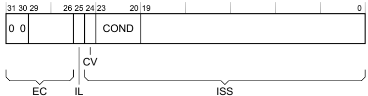
Figure G4-17 HSR format when the ISS includes CV and COND fields
